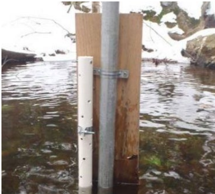
Figure 2: View of a pressure transducer attached to a metal sign.
