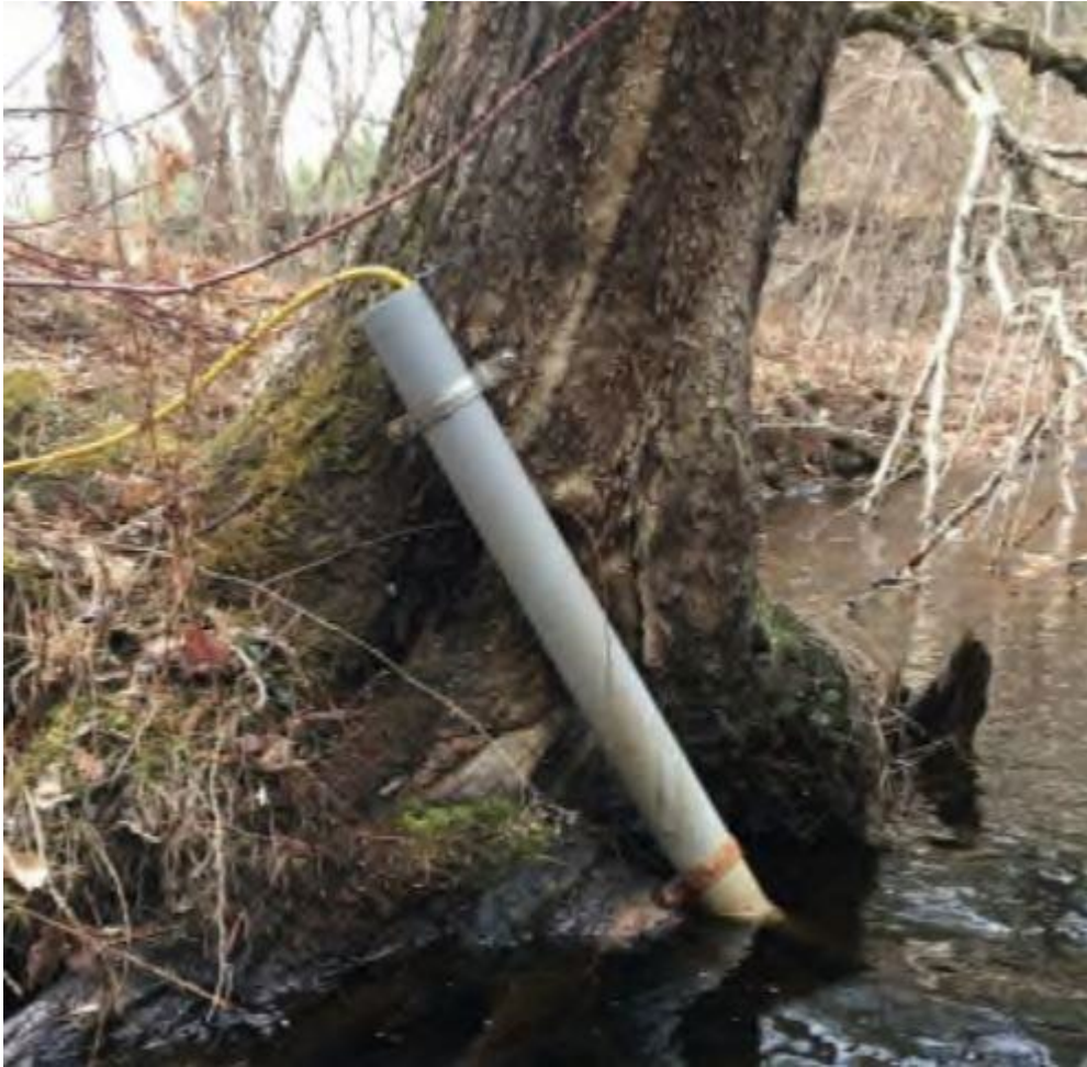
Figure 5: View of a pressure transducer attached to a tree root.
