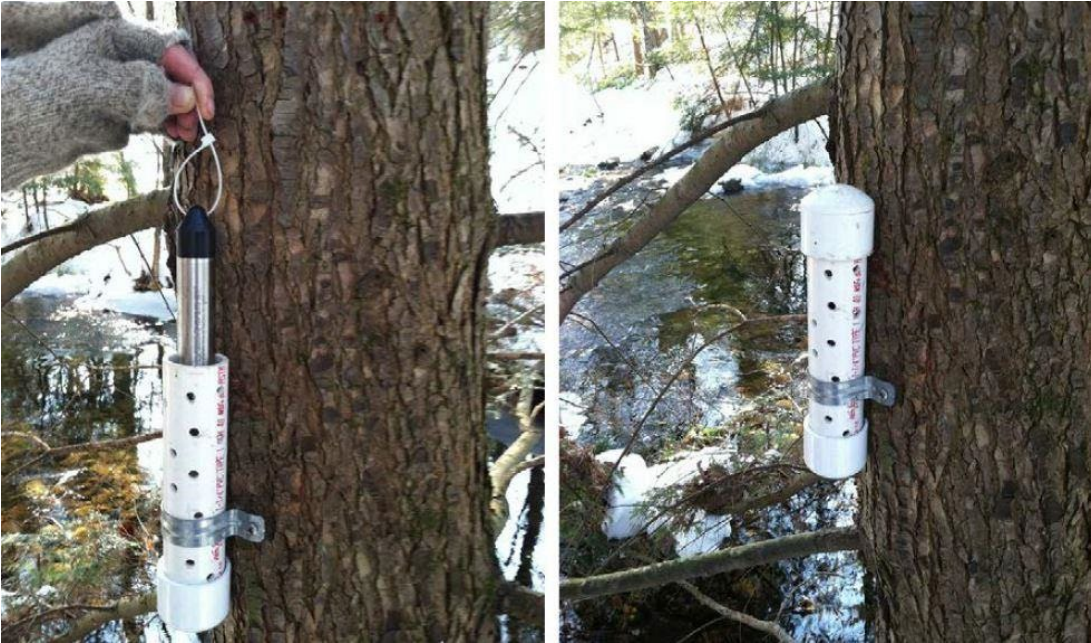
Figure 6: View of a baroTROLL® attached to a nearby tree.
